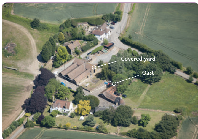
This farmstead on the North Kent Plain was developed with industrial-scale buildings in the late 19th century – the oast for drying and storing hops at the bottom of the photograph and the covered yard for fattening cattle and conserving their manure. All the buildings use locally distinctive brick and tile, and are a significant part of the local scene. Photo © English Heritage NMR 27195 010
